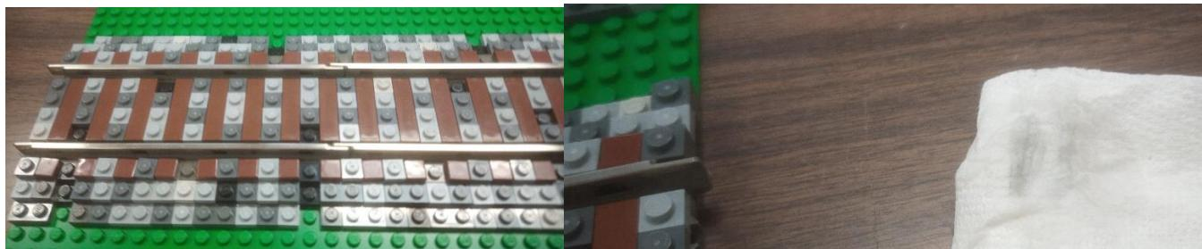
After light treatment of surface stains on the rail with 1000-grit dry sanding to bring the rail to a mirror finish, the same wiping picked up a dark stain of black gunk. The dry sanding had generated additional need for cleaning and would have spread black gunk to previously-cleaned track had a train run on it.
